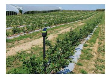
AGREUS® is a wireless system of the Smart Village class that enables the acquisition of measurement data facilitating agrotechnical decision-making and control. The system includes dedicated sensors and executive modules as well as an application available on both desktop computers and mobile devices, such as laptops, tablets or smartphones.
